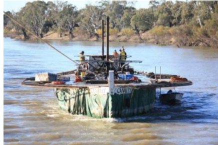
Canally under tow note the Paddle wheel frames and Shafts on the deck
